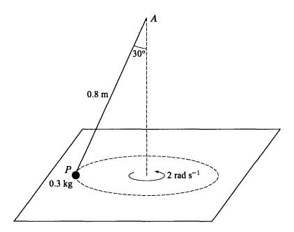
One end of a light inextensible string of length 0.8 m is attached to a fixed point A which lies above a smooth horizontal table. The other end of the string is attached to a particle P, of mass 0.3 kg, which moves in a horizontal circle on the table with constant angular speed  $2 \operatorname{rad} s^{-1}$ . AP makes an angle of  $30^{\circ}$  with the vertical (see diagram).
