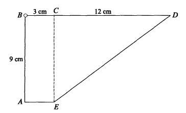
A uniform lamina ABCDE of weight 30 N consists of a rectangle and a right-angled triangle. The dimensions are as shown in the diagram.
